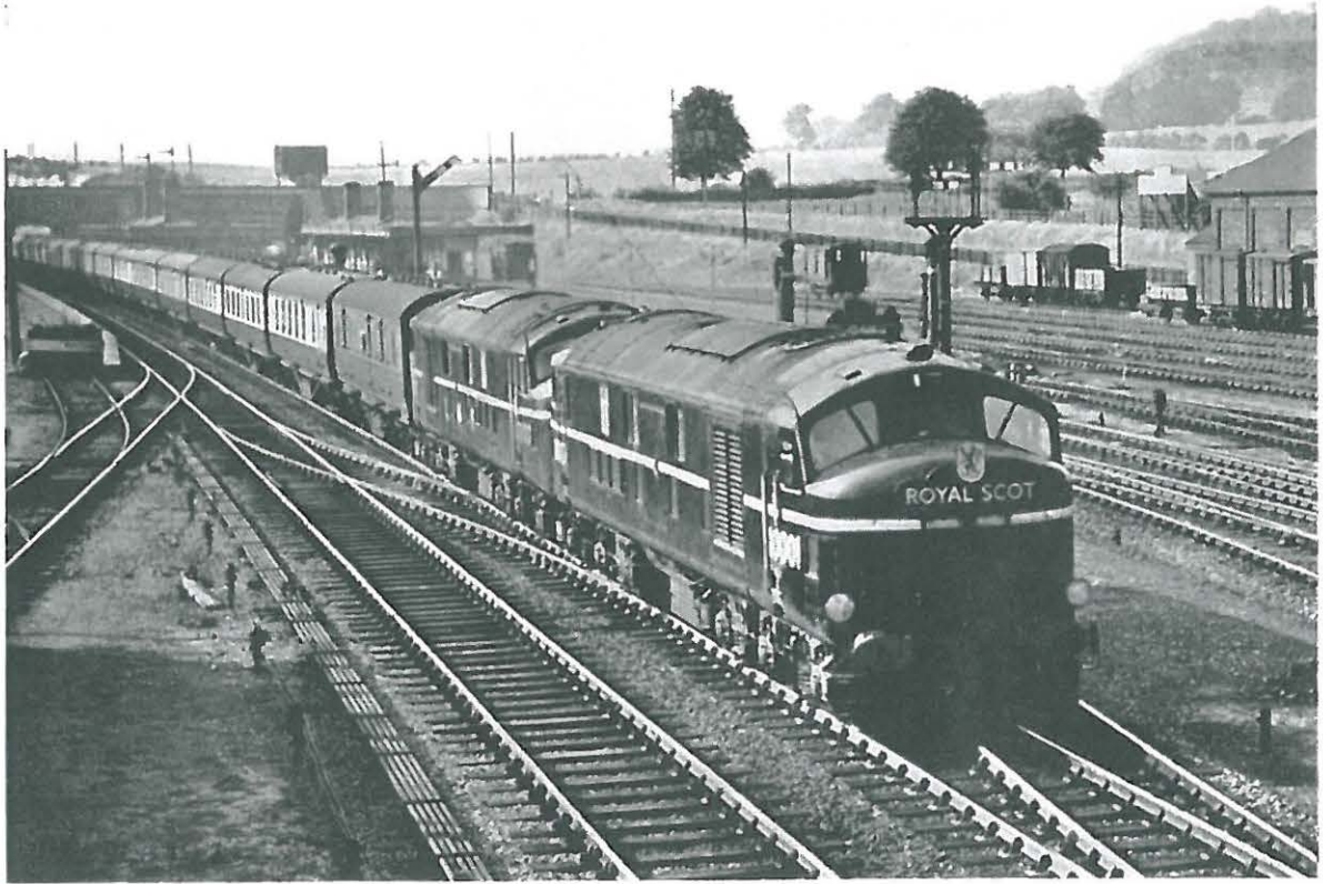
Fig. 10 Twin 1600 h.p. diesel-electric locomotives hauling "Royal Scot" Glasgow-London express
